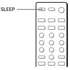
Press SLEEP on the remote while the power is on. Each time you press SLEEP, the time changes as shown below.
